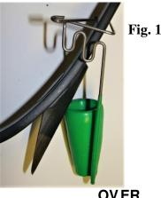
2. Slide the Gaff Guard down the climber shank, place the gaff inside the spring portion of the gaff guard and then slide the gaff guard up the leg iron shank to ensure full insertion of the gaff into the guard as shown in Fig. 2.
